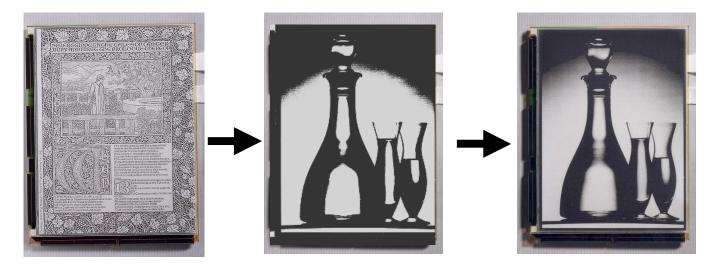
Figure 4: Image update using reset to closest rail approach: Previous image (left hand side) is switched to a reset state formed by a 1 bit representation of the following image (middle) before being driven to final image (right hand side)
