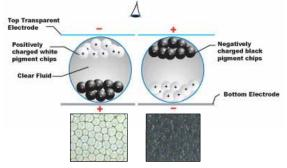
Figure 1: Electronic ink basic principle
